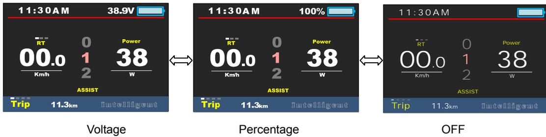
**8.6 Clock** : Clock setting, press **MENU** button get into the clock setting menu, press UP/DOWN button to set Year/Month/Day/Hour/Min/Sec.
