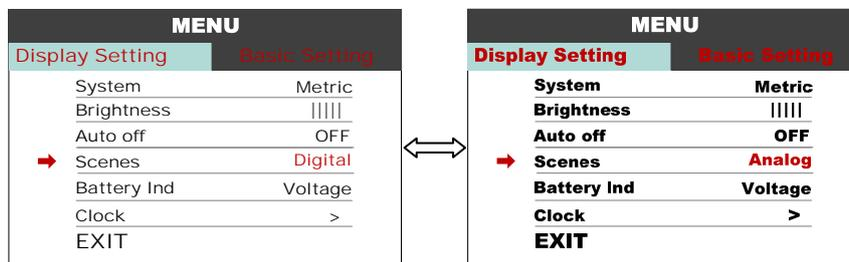
**8.5 Battery Ind** : Press UP/DOWN button to change the battery indicator, Voltage / Percentage / OFF.
