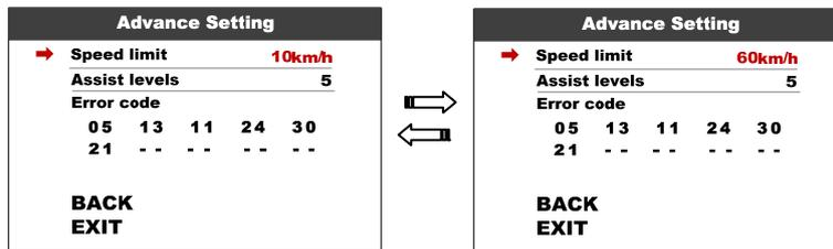
**8.12 Assist levels:** This parameter can customize assist levels, options are 3/5/9/UBE, UBE represent factory default settings.
